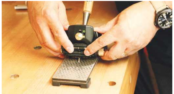
▲ The roller has micro adjustments to set a honing bevel if required
